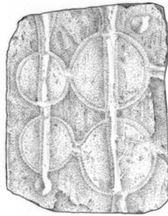
Sketch 2. Slate molds for producing lead disks (designed by E. Theou)
