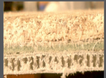
Cross section of a conserved detached wall painting lined with a 3D fibreglass fabric support.
